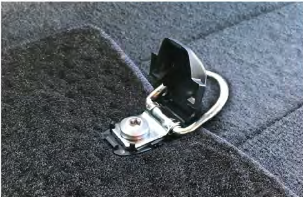
Step 5. Reinstall the tie down to secure the Cargo Gap Mat.
