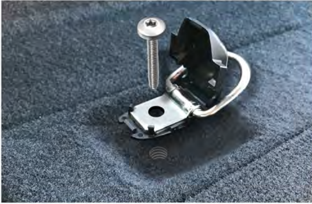
Step 2. Unscrew the Torx screw and remove the tie down.
