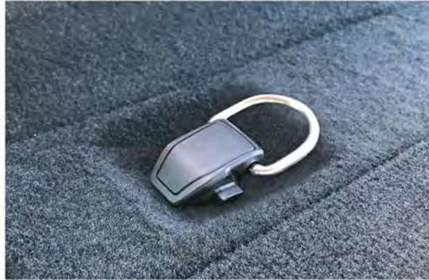
The floor tie downs used to secure the Cargo Mat are located just behind the rear seats.
