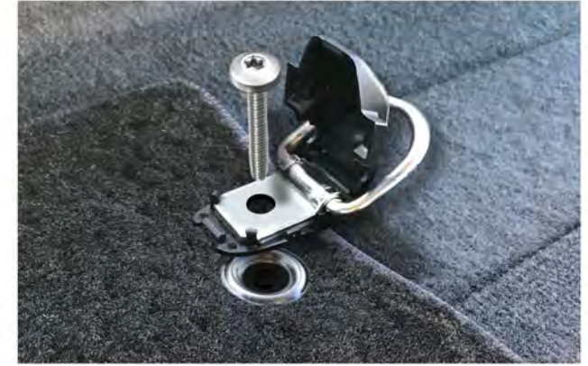
Step 4. Place the tie down over the Cargo Gap Mat and insert the Torx screw.
