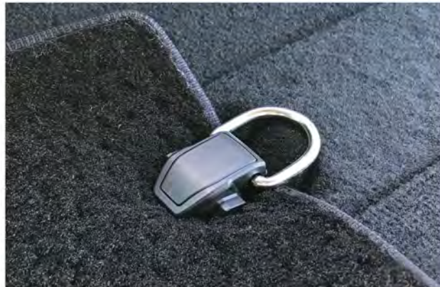
Step 6. Close the plastic tie down cover and repeat for other side.
