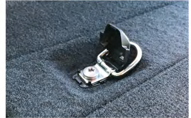
Step 1. Flip open the plastic cover on one of the tie downs.
