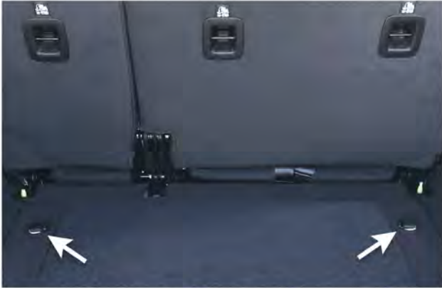
Locate the OEM Floor Tie Downs used for Cargo Gap Mat installation.
