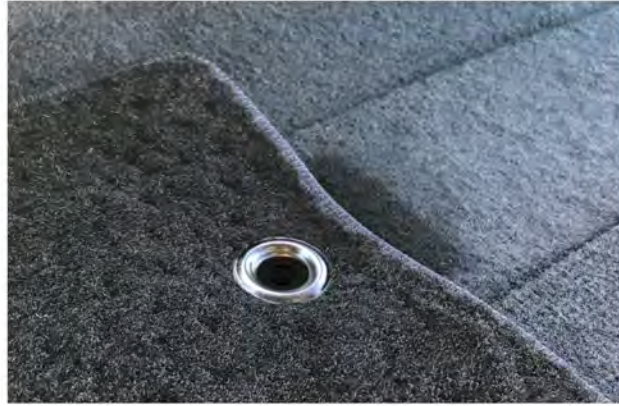
Step 3. Align the Cargo Gap Mat grommet with the threaded hole for the tie down.
