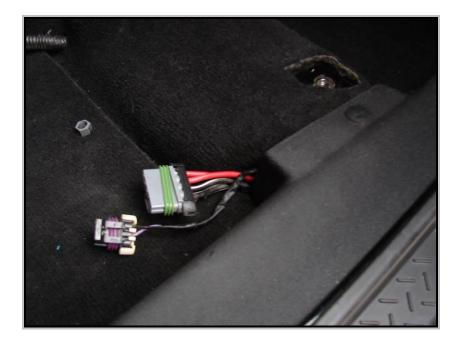
5-A) Reinstall the seat and torque the 4 bolts to manufacturer specifications (45 ft-lbs). Attach harness to compressor. Side panels are removed from the seat frame in picture below just for demonstration purposes.
