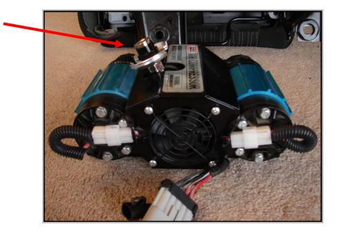
1-B) Use two of the provided wires ties to secure the main power plugs up against the compressor body and trim ends of wire ties. This is important for clearance as these wires will be close to the seat frame once the compressor is installed.
