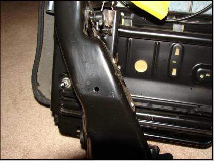
2-E) Use one of the provided wire ties to secure the two black cables as shown below. Be sure to leave the wire tie loose as shown. The cables need to be free to move as the seat is adjusted. The wire harness to the yellow plug should be between the two cables and the bottom of the seat as shown in second picture.
