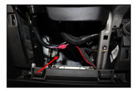
6-E) If you want your ARB switch to light up when your parking/headlights are on for visibility at night, connect the <u>blue wire w/ white stripe</u> to the <u>orange wire</u> <u>w/gray stripe</u> using the provided red T-Tap Set as shown below. The wire is located in the harness that goes to the window control module.
