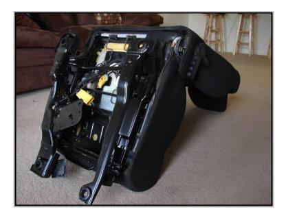
2-D) Use a drill to drill out the two rivets holding the metal plate on the bottom of the seat (on some models these may be screws, check first). You do not need to drill completely through. Just enough for the rivet heads to come off. Remove and discard, the plate is no longer needed.
