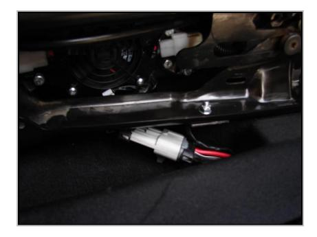
5-B) Reconnect yellow plug under seat. While looking under seat, check for clearance on wires, cables, plugs, and compressor as the seat is moved forward and back and folded and tumbled.
